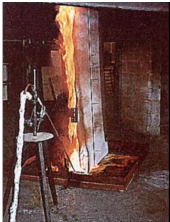
Photo 1. Polystyrene Jointed Panel Test
